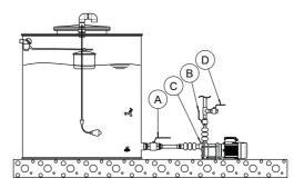
Figure 7: Example: installation of a pump under pressure operation
