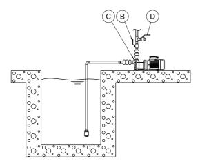
Figure 8: Example: installation of a pump in suction-operation
