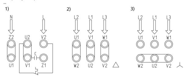
Figure 6: Wiring diagram, depending on selected motor
